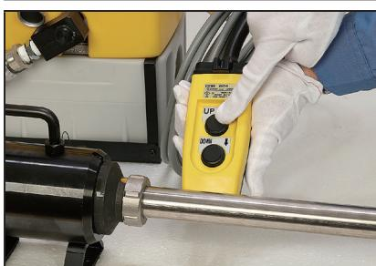
5. For the pipe expansion work, keep pressing "UP" button until the motor stops. Then, pressing "DOWN" button around two seconds to release the pressure.
