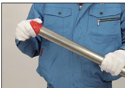
2. Carefully, remove burrs from both the inner and outer chamfered surfaces carefully using reamer, sand paper and grinder.
