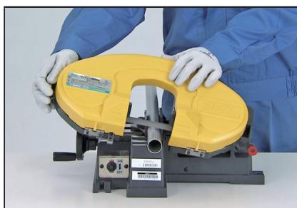
1. Referring to the pipe cutting dimension table, cut the pipe at a right angle to the axis core with a metal saw or band saw.
