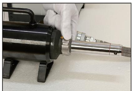
3. Tighten the cap nut to the yoke.
