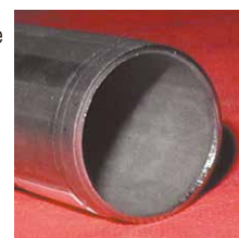
After burrs are removed with a reamer
